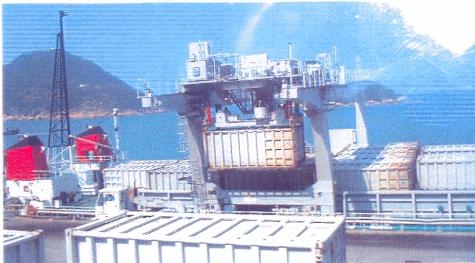
After pulverizing & compacting the garbage to 1/3 the original size, it is then loaded onto ship to be shipped to land fill site around designated site to be used as land fills. The most amazing thing is that no odor or waste water can be detected from this complete peration.
