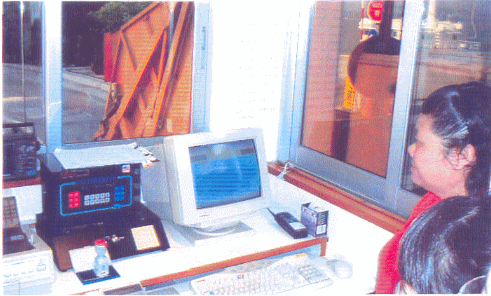
At the entrance of the plant are weighing machine to check the trucks coming in and going out to tally the amount of garbage being passed through the gate.
